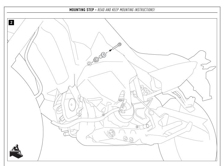
Remove the screw shown on the left side of the vehicle.
