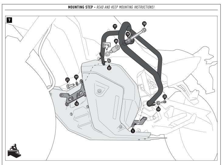
Screw the left half of the crash bar (17) to the mounting bracket (1), to the cross connector (13), and to the original damper (Orig.) on the vehicle.
