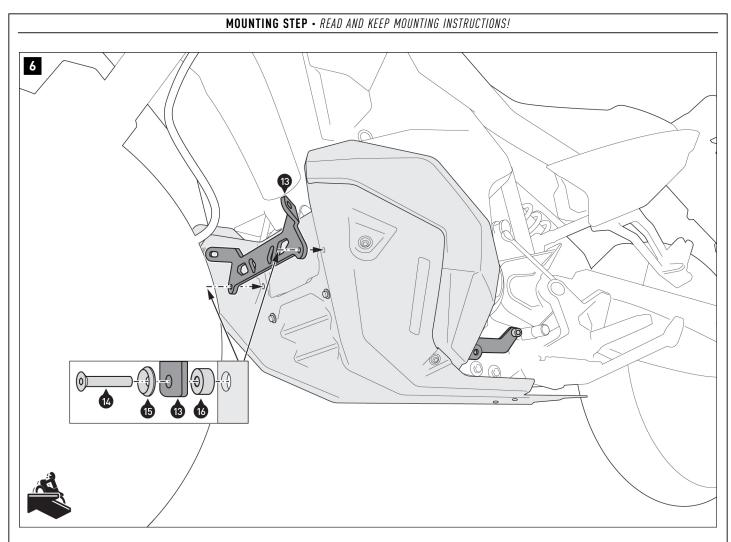
Reattach the original engine guard to the vehicle. **A WARNING: Use a liquid threadlocker!** Tighten the original screws according to the manufacturer's instructions.
